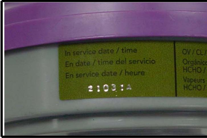
The photograph above shows the date code from a Survivair model 1058 cartridge. It illustrates the location of the date code on the label. The third and fourth digits from the left in the code pictured above indicate the year that the cartridge was manufactured. The 03 in 21031A indicates that the cartridge shown in this photograph was manufactured in 2003. We are looking for cartridges manufactured in 2002 and therefore are looking for cartridges marked with 02 stamped in this location.
